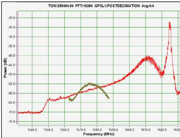
**Figure 14 Power Spectrum Pre-Decimation (red) and Post Decimation (green) View with Out of Band Narrowband Interference**
